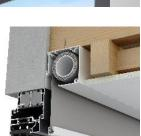
A headbox is a metal recessed box in which the roller blind is mounted. They can be installed inside or outside the window recess, but they are normally installed into a ceiling recess, fitted flush with the ceiling surface.
